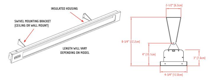
Heater must be installed with the quartz tube horizontally level. For maximum tube life, use a level to find the optimum position for the heater's body. Always maintain the minimum clearances from the heater body to any combustible materials.
